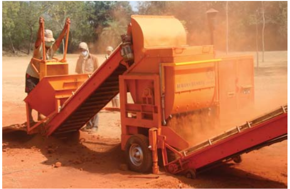
Filling the Auram Crusher's hopper with wheel barrows
