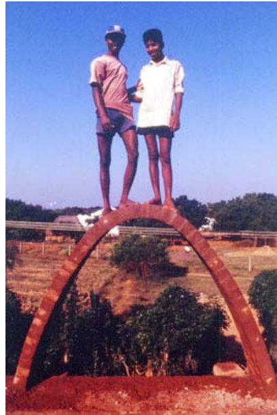
Testing a catenary arch of 2 m span
