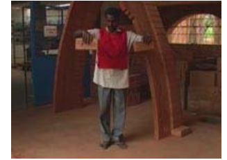
Comparative strength of a half size plain CSEB and a fired brick
