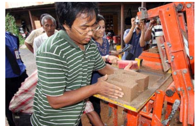
Producing blocks with indent for vertical bars
