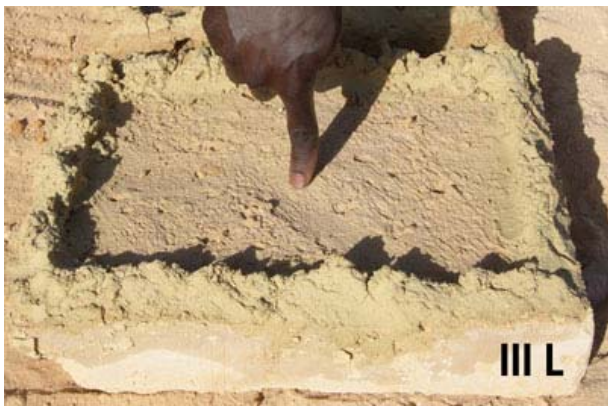
Excellent result of absorption test with lime stabilisation
