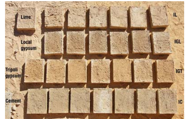
Series of test with various stabilisers
