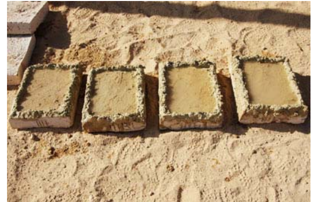
Absorption test on stabilised adobes
