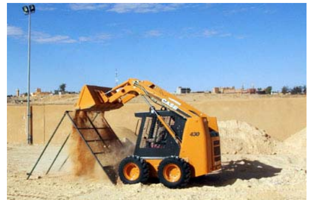
Sieving soil with the dumpy loader
