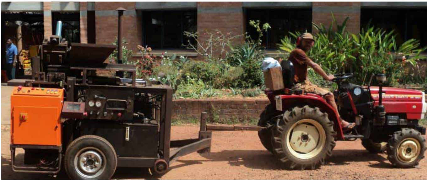
The Auram 6000 hydraulic press fully assembled and pulled by a tractor
