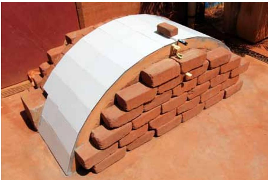
*Vaulted structure with tiles ready for testing*
