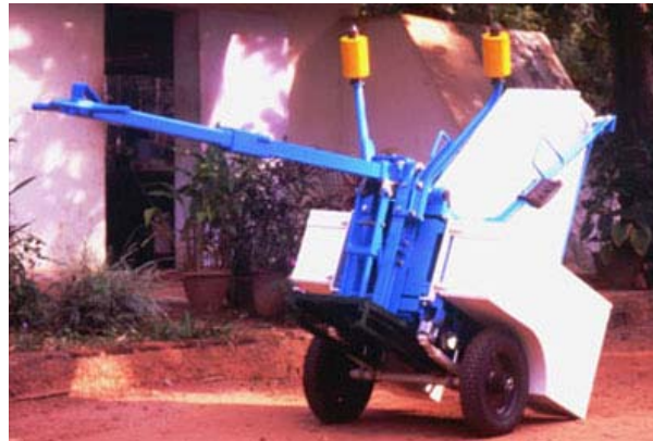
The Auram press 3000, on a wheels for road transportation
