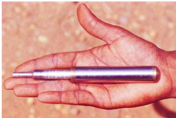
Pocket penetrometre ( 5 kg/cm 2 ) for checking the compression quality of freshly compressed blocks
