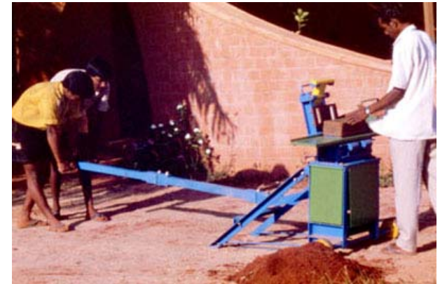
Auram presses 240, 290, 248 or 298 - Single mould manual presses Note that these presses are not produced anymore
