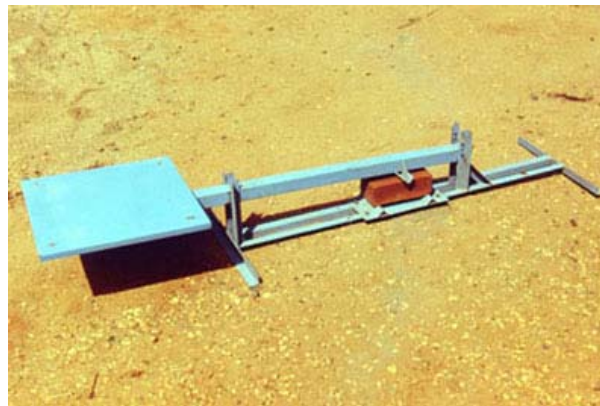
Field block tester for testing the bending strength of blocks
