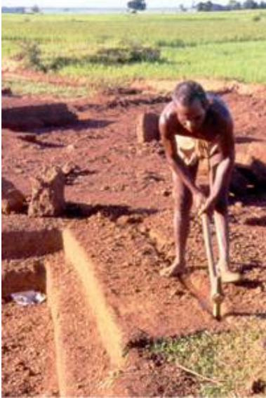
India, Orissa, Near Narangarh – Cutting petroplinthite by hand
