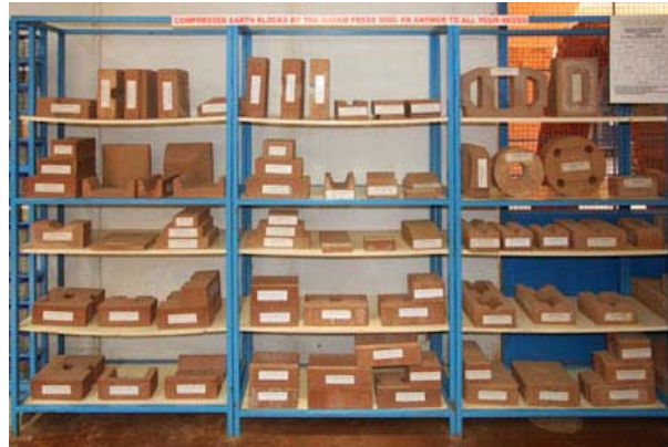
About 75 different blocks produced by the Auram Press 3000
