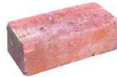
Wire cut fired brick (22 x 10.5 x 7.2 cm)
