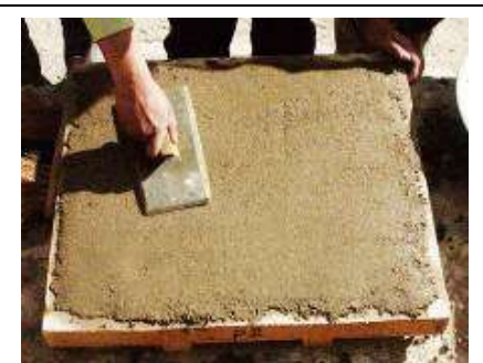
10. Pressing the coats with a wooden float
