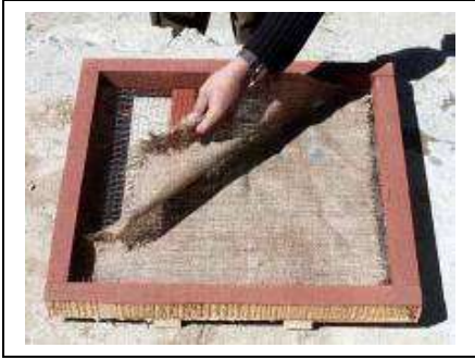
1. Frame, mesh and jute clothe
